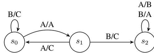
Fig. 3. A Mealy machine with 3 states
